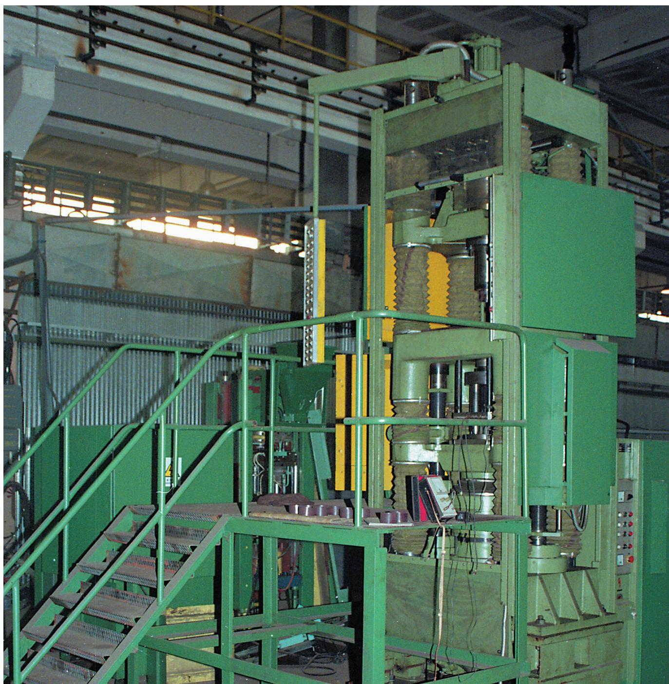
**The PXP presses**, which are of original Polish design, form parts from powders and sintered pre-forms by means of an innovative pulsatory pressing technology. This method imposes a quasi-static force with a rapidly changing frequency, reaching several hundred hertz. As a result of this method the pressing load and ejection force are reduced. This method also improves product density and its homogeneity, as well as, eliminates part cracking.
