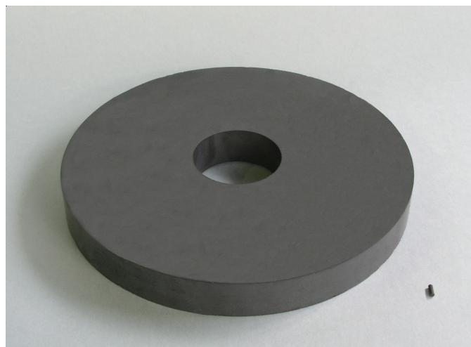
Drawing of a ring with radial anisotropy for an electric motor and isotropic sleeve for a resonator for persons with speech impediments
